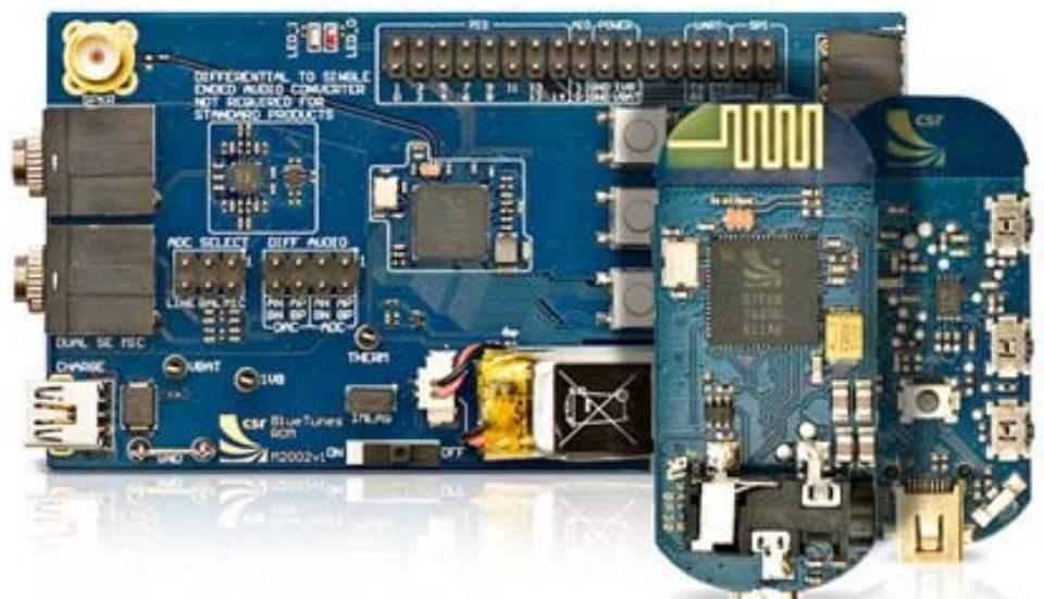
*The BlueTunes ROM headphones design (both sides of example design, and the development board shown) exploits the ROM-equipped variant of CSR's highly integrated BlueCore5-Multimedia device. Based on an 8x8 mm QFN packaged device and just a few additional components, the design offers significant component savings compared with previous Flash-based solutions.*
