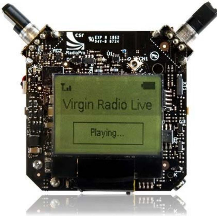
CSR's 2-chip internet radio design can be implemented in a very small form factor, as this demonstration hardware shows (it measures 5x5 cm and that's with just a single-sided PCB). Tools allow users to customise the user interface, and hardware elements such as the user interface.
