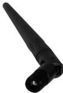
The CTi-SB series of stubby ZigBee antennas comprises three models, with a choice of straight and right-angle SMA male and SMA male RS connectors. For applications that demand increased signal strength, the slightly longer CTi-RA series of rubber ZigBee antennas provide a gain of up to 9 dBi. These antennas employ co-linear elements - contained within a semi-flexible rubber housing - to maximise RF efficiency, and
