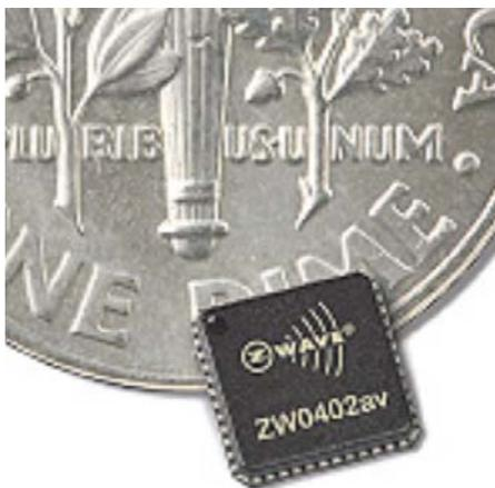
Figure 1: Zensys' Z-Wave System-on-Chip Solution.
